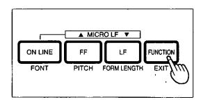
Press FUNCTION (EXIT) to exit the FUNCTION mode.
