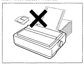
Do not obstruct the movement of the printhead while in operation.
