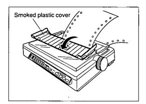
Fold the smoked plastic cover forward by lifting tab on right side.
