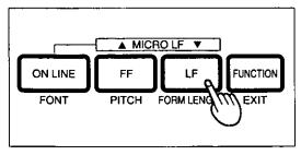
Press and release **LF** (FORM LENGTH) to reach the desired form length.
