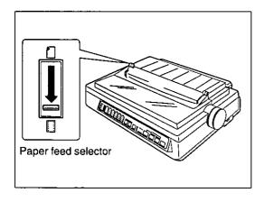
Move the paper feed selector to " [i] " (Push Tractor mode).
