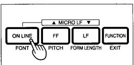
Press and release ON LINE (FONT) to reach the desired font. Go to step 4.
