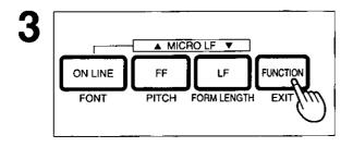
Press FUNCTION (EXIT) to exit the initial setup mode.
