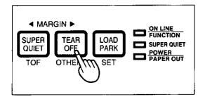
Press and release <u>TEAR OFF</u> (OTHERS) until the column indicator is blinking over FACTORY.
