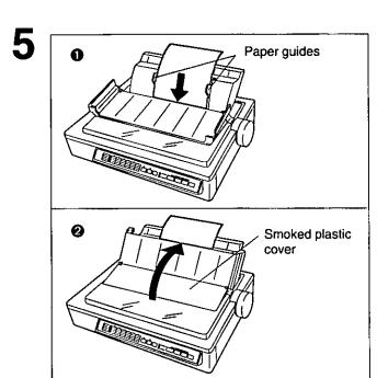
• Insert a sheet of paper through the paper guides and behind the platen.
