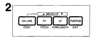
While pressing FUNCTION, press LF to clear the data in the receive buffer.
