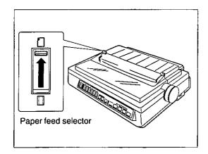
Move the paper feed selector to " [ " (Friction mode).
