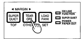
Press TEAR OFF to advance the paper's perforation to the tear bar.
