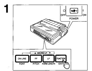
While pressing **FUNCTION**, turn the power switch on.
