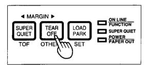
Press and release **TEAR OFF** (OTHERS) until all the column indicators are blinking.
