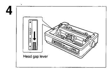
Move the head gap lever to the (+) position.
