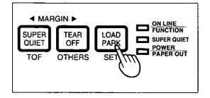
Press LOAD/PARK to reload the fanfold paper to the Top of Form.
