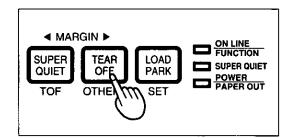
Press and release TEAR OFF (OTHERS) until the column indicator is blinking over the desired margin.
