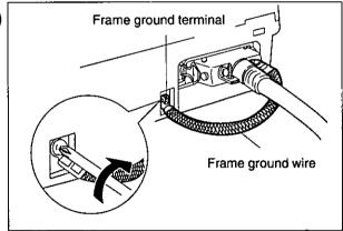
If the cable has a frame ground wire, connect it to the frame ground terminal.
