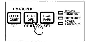
Press and release <u>TEAR OFF</u> (OTHERS) until the column indicator combination is blinking over your desired color.
