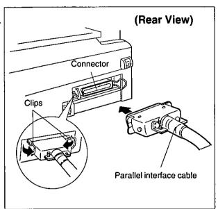
Attach one end of the parallel interface cable to your printer as shown, and the other end to your computer.
