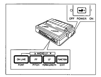
While pressing both **LF** and **FF**, turn the **power on**.
