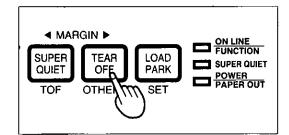
Press and release TEAR OFF (OTHERS) until the column indicator is blinking over COLOR (OPTION).
