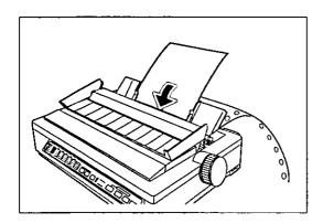
Separate the paper guides and load a single sheet or an envelope.
