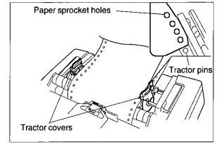
Align the paper sprocket holes with the tractor pins.
