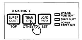
Press and release <u>TEAR OFF</u> (OTHERS) until the column indicator is blinking over MACRO #1 or #2.
