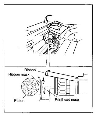
Slip the ribbon between the ribbon mask and the printhead nose.
