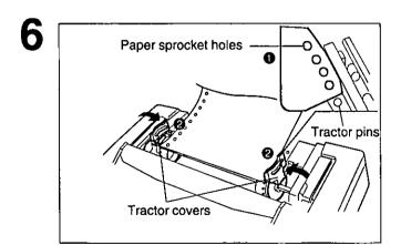
To set the tractors to the proper width, align the paper sprocket holes with the tractor pins by moving the tractors.
