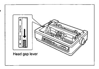
Move the head gap lever to the (+) position.
