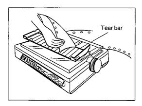
Tear off the page, using the tear bar.
