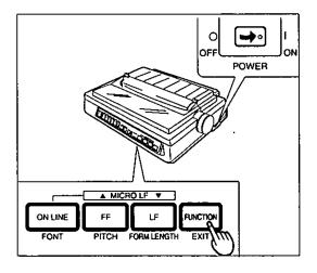
While pressing **FUNCTION**, turn the power switch on.
