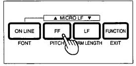
Press and release FF (PITCH) to reach the desired pitch. Go to step 4.
