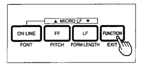
Press FUNCTION (EXIT) to exit the FUNCTION mode.
