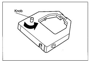
Rotate the knob on the ribbon cassette to remove any slack.
