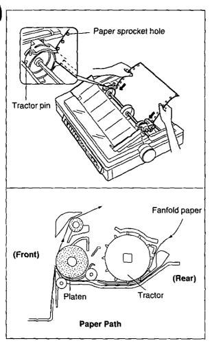
While the tractors are rotating, insert the fanfold paper evenly behind the tractors, until the tractor pins catch the paper sprocket holes.
