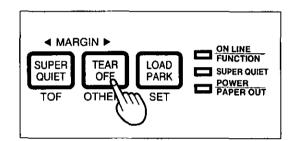
Press and release TEAR OFF (OTHERS) until the column indicator is blinking over MACRO #1 or #2.
