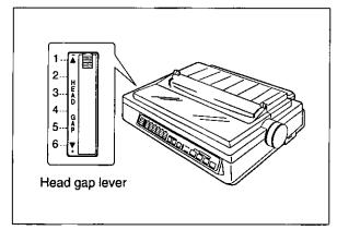
Adjust the head gap lever for the thickness of the paper you are using.
